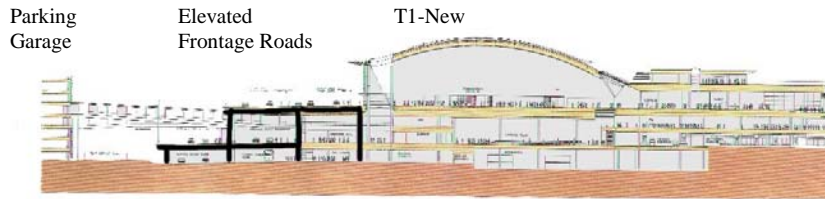
Figure 1 – General arrangement of Elevated Frontage Roads
